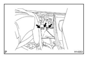
(b) Install side gate seal with the clip.
